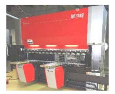
Installed at the front of the machine and supports sheets. The operator need not support sheets. When sheets are particularly heavy, the fatigue of the operator is lessened throughout the bending operation.
