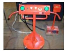
A stand-type control device with two-hand control pushbuttons.
