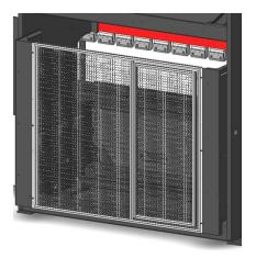
Prevents entry from the rear of the machine. The rear guard reduces the risk of the operator getting the hands pinched between the punch and die or getting impacted by the backgauge.
